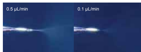
Change in Spray Shape at Different Flow Rates
